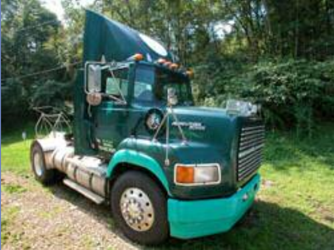
1995 Ford L-9000 s/a tractor, VIN: 1FTYS96U7SVA03271, Cummins N14 400 hp engine, 21200 lb. rear axle, 530000 mi. on odometer
