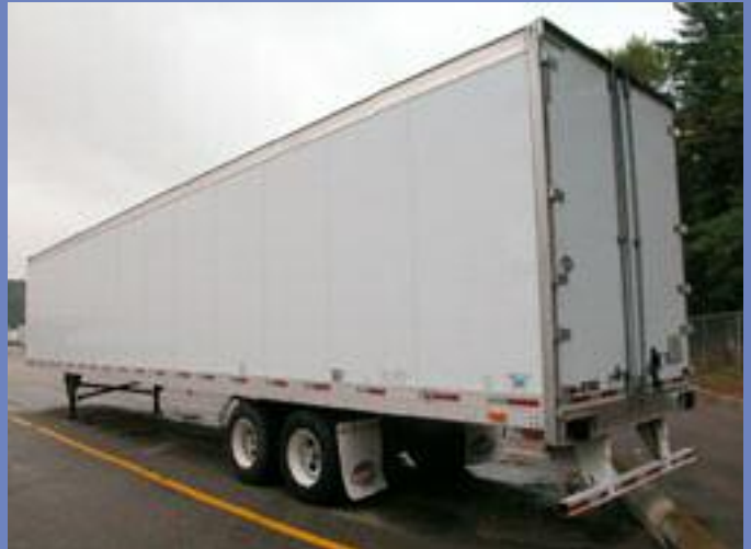
2003 Utility 53' alum. dry van trailer, Model VS2DC, VIN: 1UYVS25333G097612, tandem slider, air suspension, swing doors
